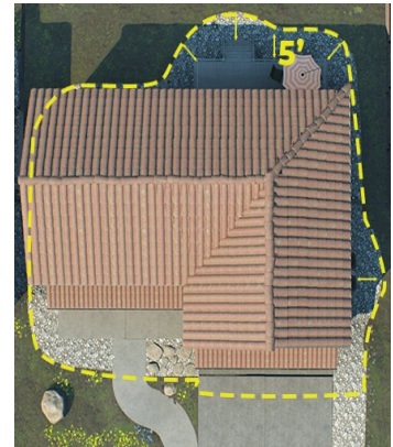
During a wildfire, embers can travel miles ahead of a fire front and accumulate at the base of your home's exterior walls and within the first 5 feet. By implementing a buffer zone, you significantly reduce the chances of your home being ignited by wildfire.
