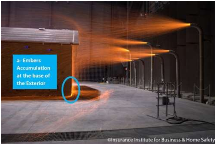
Figure 1. Ember accumulation at the intersection of exterior walls and ground [2].
