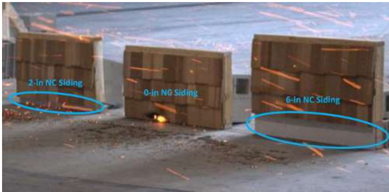
Figure 3. Accumulation of embers at the base of the exterior walls.
