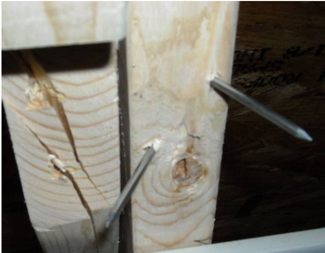
Figure 15 – Nail withdrawal and pull-through failure modes of 16d nails
