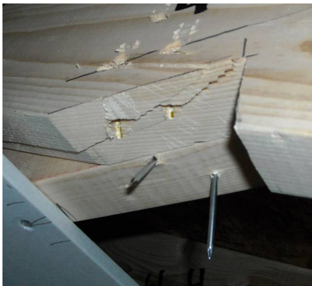
Figure 14 – Nail withdrawal of the 8d nails and pull through of 16d nails
