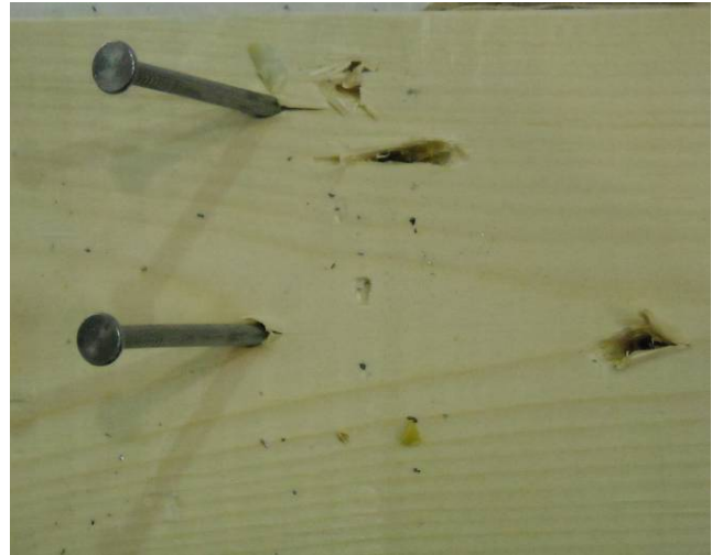
Figure 16 – 16d nails in plate after pull-through failure
