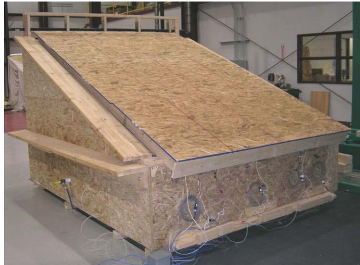
Figure 5 – Uplift specimen ready for testing
