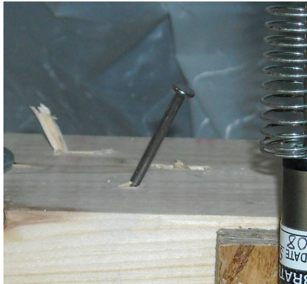
Figure 13 – Nail after pulling through rafter
